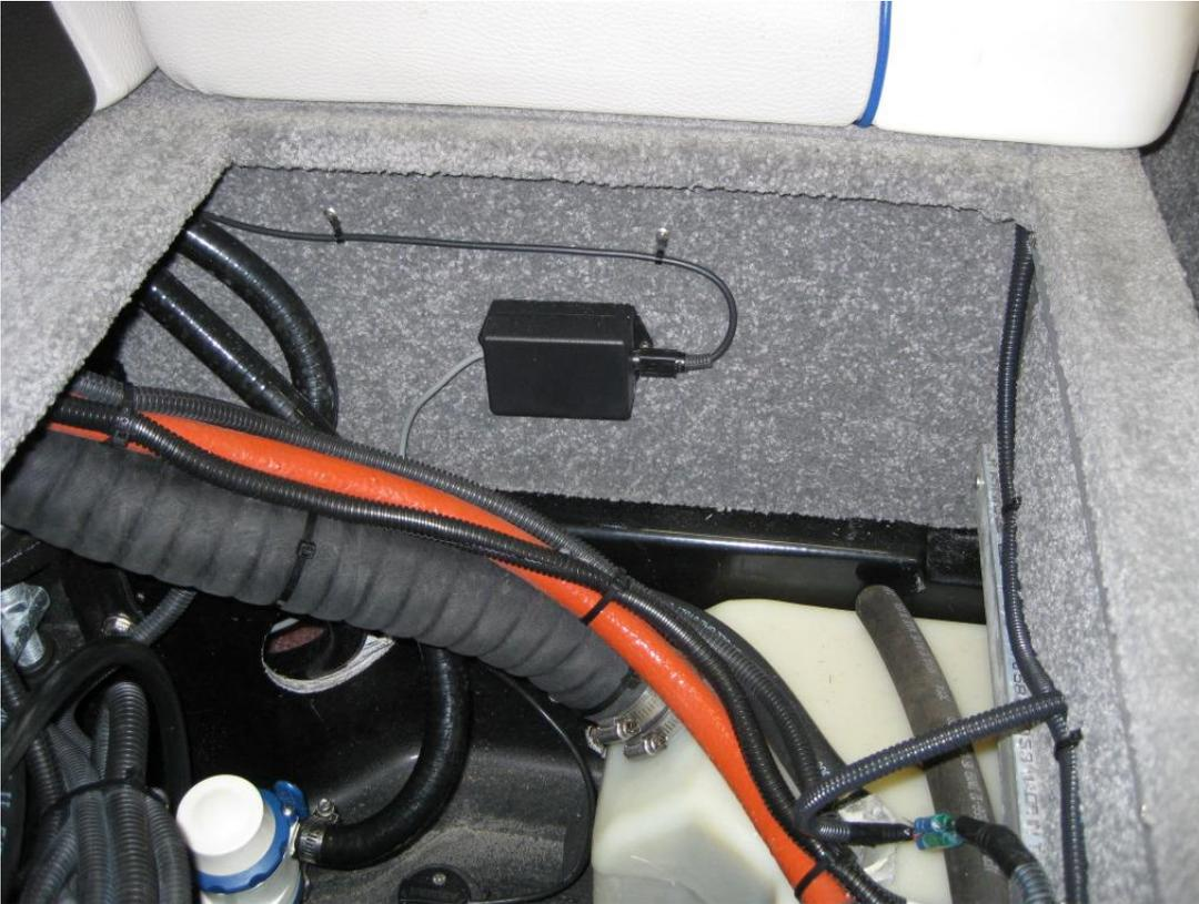
I ran my GPS cable up along the port side of the boat and mounted the Garmin puck right in front of the glove box.
