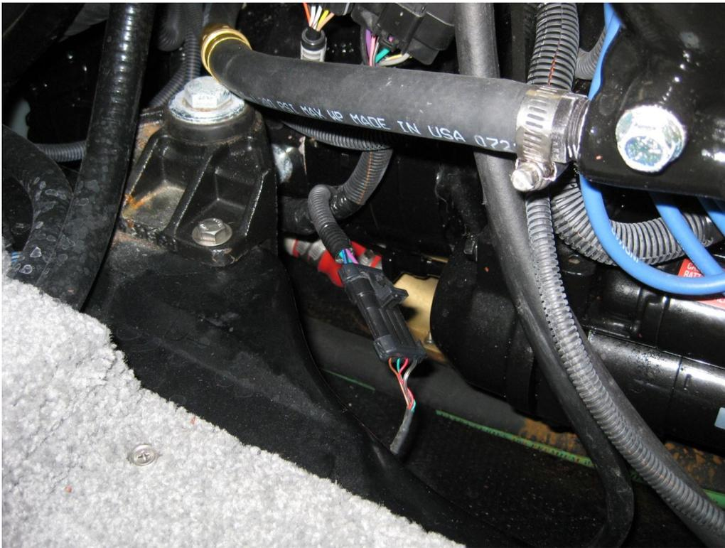
Disconnect the 4 pin plug that plugs your paddle wheel into the boats harness, connect the mating plugs from the NL4 harness to the plugs that you just disconnected as shown here.
