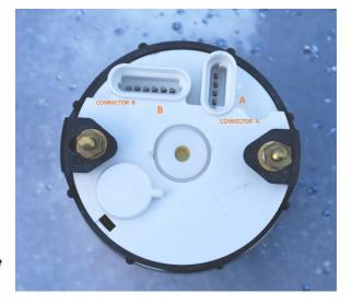
Insert the loose wire harness Connector A (Delphi Socket) into the NL4-Fc's Delphi 4 position Plug Connector. THE LATCH ON THE Socket CONNECTOR SHOULD FULLY ENGAGE THE RAMP ON THE Plug CONNECTOR.
