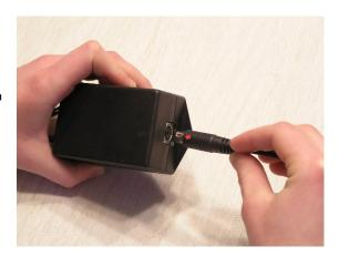
On a 'cold start' (power turned on after a prolonged off period) the GPS Receiver may require 1 - 2 minutes to sync to the satellites. With a warm start, expect the satellite sync within seconds.
