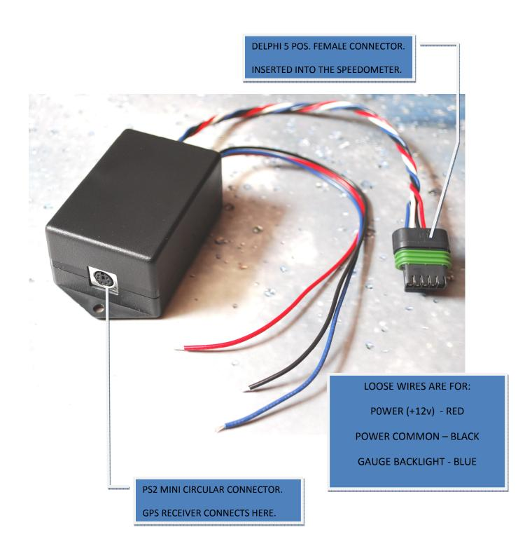
The installation of the NL3 and Speedometer is not complicated. The process is analogous to installing a car stereo. Before you begin, have a clear idea/plan of where to tap the boat's +12Vdc power, common, and dash lights; please refer to manufacturer, local dealership, mechanic, and/ or online manuals for greater insight.
