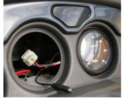
connector, and accomplished this without breaking the connector, clip, or speedometer. Otherwise, the gauges are secured with a rear mounting bracket. The bracket is captivated by two nuts (5/16ths). Remove the nuts. Slide the bracket back and clear of the screws. Pull the gauge out of the dash front, Remove the connector by lifting the connector latch up, while backing it out.
